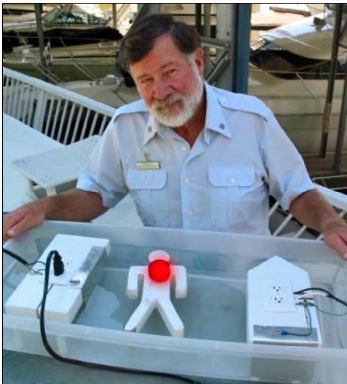
John Hardin demonstrates his ESD training aid that depicts leaking electricity that can cause paralysis. A large red bulb on the figure lights up to indicate the presence of stray electrical current.
