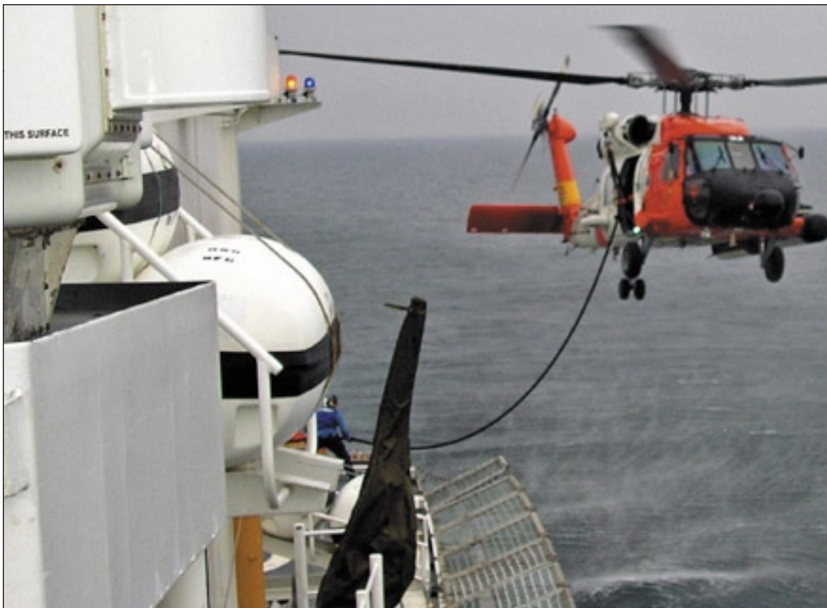
One of the activities of great interest to Auxiliarist Jerry Janaro as he cruised on USCGC Escambia with his son, LTJG Jeff Janaro, was Helicopter In-Flight Refueling. HIFR is a method of extending the flight duration of Coast Guard helos by hoisting up a HIFR rig and pressure-refueling from HIFR-capable Cutters. The helo seen here is from USCG Air Station Cape Cod.
