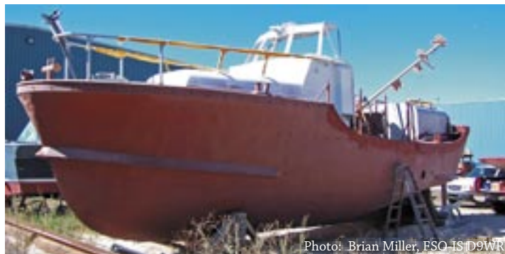
The work-crew for the MLB-44 sand-blasted everything – including the windows, unfortunately! – right down to bare metal, then primed her.
