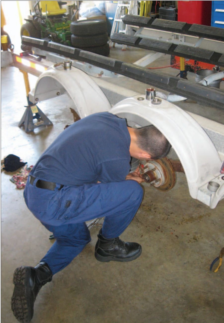
JD DeCasta, mechanical engineering senior at Auburn University, repacks the wheel bearing on a Coast Guard boat trailer at Station Dauphin Island.
