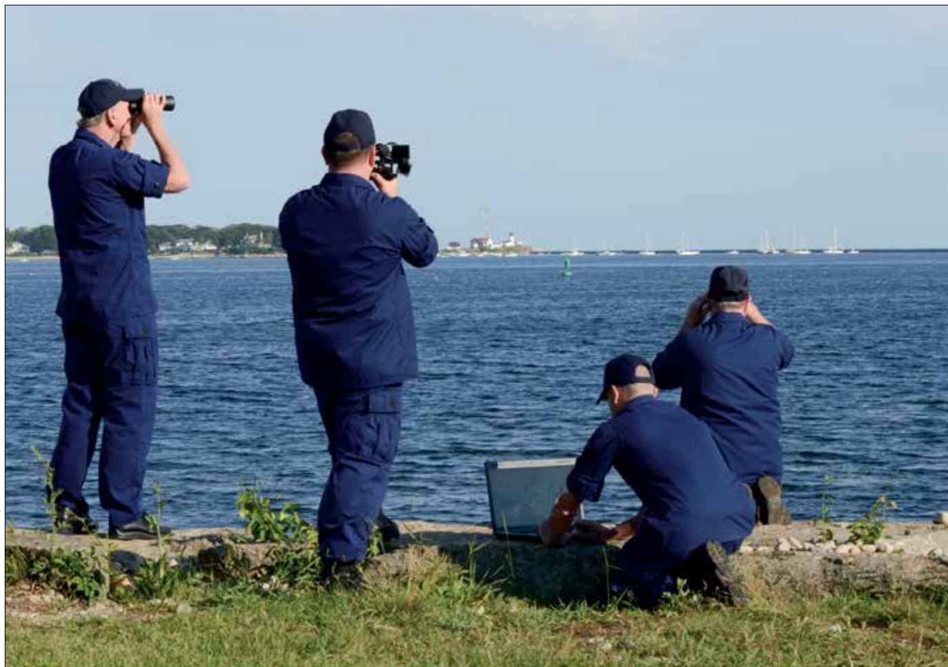
The First Northern Division Four ATON/Waterways survey team working Gloucester Harbor, Gloucester, Massachusetts, in April 2013. Left to right are Ken Wilson, Flotilla 41, Beverly, waterways scanning; John Keyes, Flotilla 46, Cape Ann, taking the horizontal angles with a sextant; Mike Bergmann, Flotilla 46, entering the data; Kevin Meagher, Flotilla 41, with the laser range finder.
