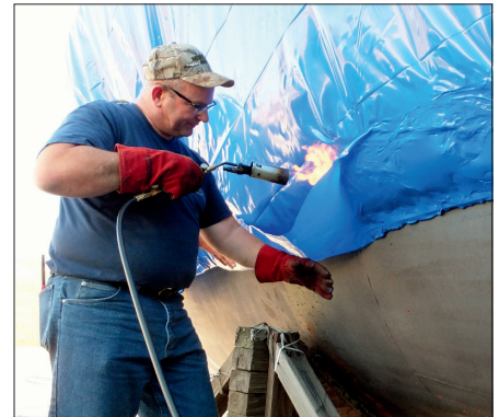
MUSKEGON — Coxswain Ken Bennett applies heat to the shrink-wrap of Aux 44359 to make it secure to nylon banding around the hull.
