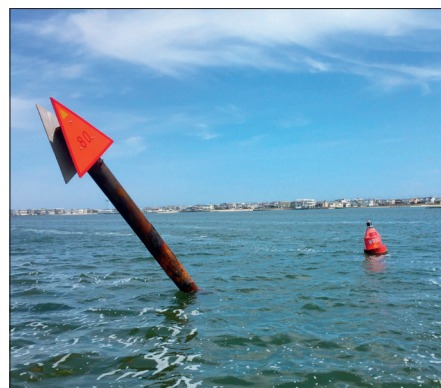
A leaning day beacon is marked with a temporary lighted beacon. .
