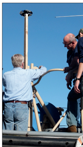
MUSKEGON — Auxiliaries Ken Bennett and Tom Johnson construct a frame on Aux 44359 that will support shrink-wrapping during winter lay-up.
